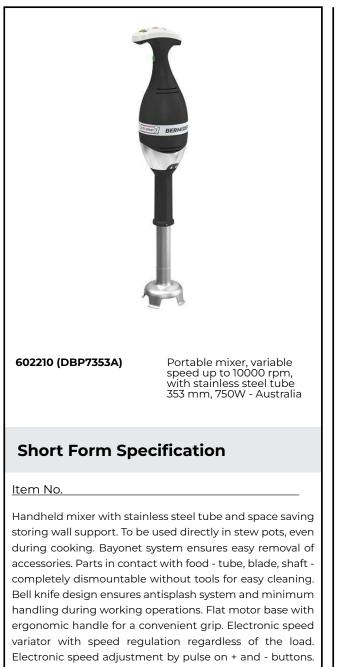
variator with speed regulation regardless of the load. Electronic speed adjustment by pulse on + and - buttons. Maximum speed: 10000 rpm. Safety feature requires both hands to start the machine. Design for heavy duty usage: double fan system to cool down the motor. Visible and water proof (IP55) control panel to control speed levels and overload warning light. Shaft locking device avoids release during operation. Whisk accessory available as an option.
